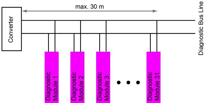
Figure 5.4: Stylized view on the Diagnostic Bus
