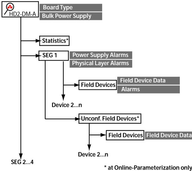
Figure 8.17: Menu structure HD2-DM-A
