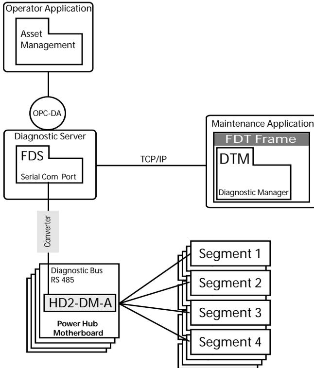
Figure 5.1: Schematic structure HD2-DM-A, see legend below
