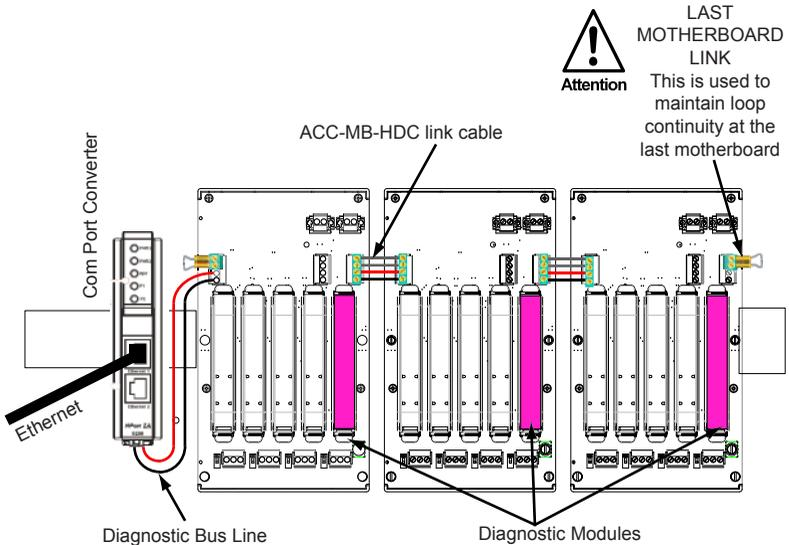
Figure 5.5: Cabinet installation example with Ethernet/RS 485 converter
