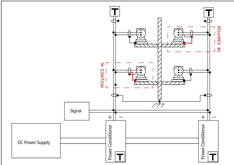
Figure 9.3: Fault wiring DC unbalance
