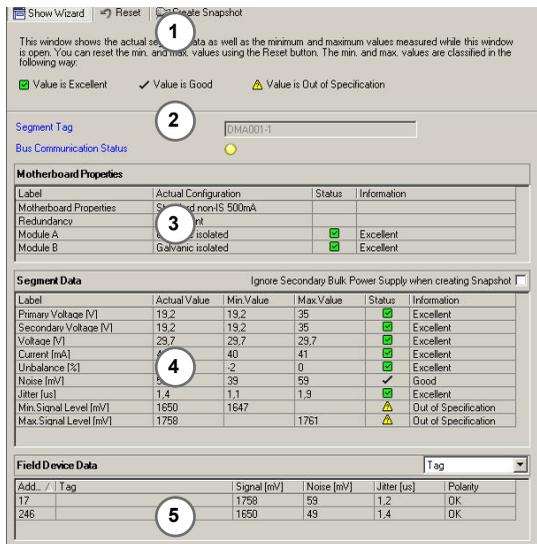
Figure 8.6: Segment Monitoring function screen overview
