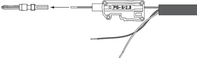
4. Solder up the lead within the Metal Part.
