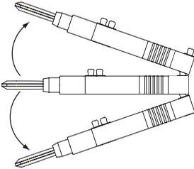
2. Remove the Metal Part from the Test Plug.
