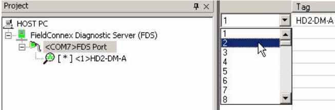
Figure 5.16: Device address settings
