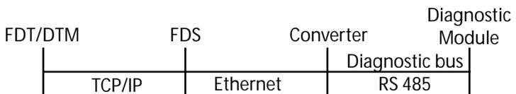
Figure 5.3: Remote application data flow
