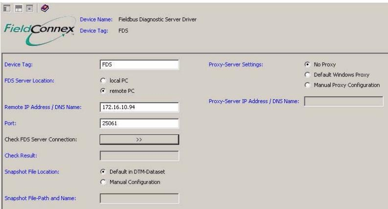
Figure 5.20: Fieldbus Diagnostic Server Parameter window
