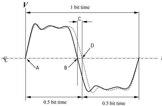
Figure 9.2: Bit cell jitter
