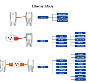
In Ethernet Mode, SignalTEK II FO connects with copper or fiber cable
