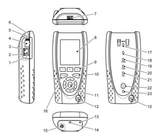
SignalTEK II shown with Power Module item 13 fitted. When Battery Pack is fitted, items 14 & 15 are not present.
