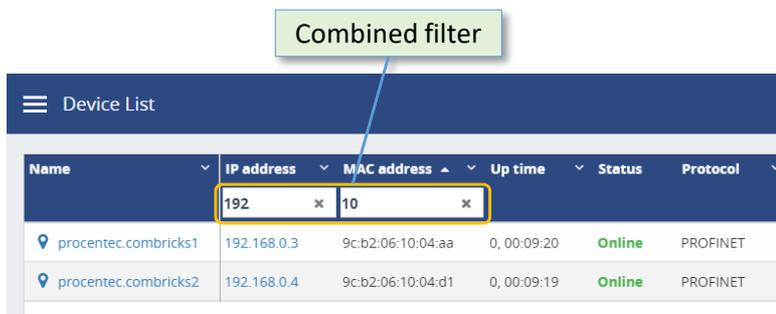
Figure 20 – Combined IP and MAC address filter
