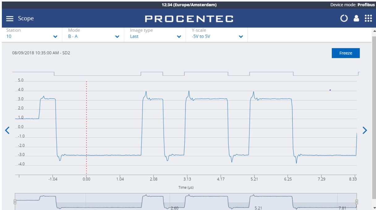
Figure 26 – Normal oscilloscope image of device 10
