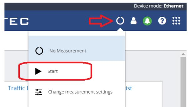
Figure 12 – starting a measurement in web interface
