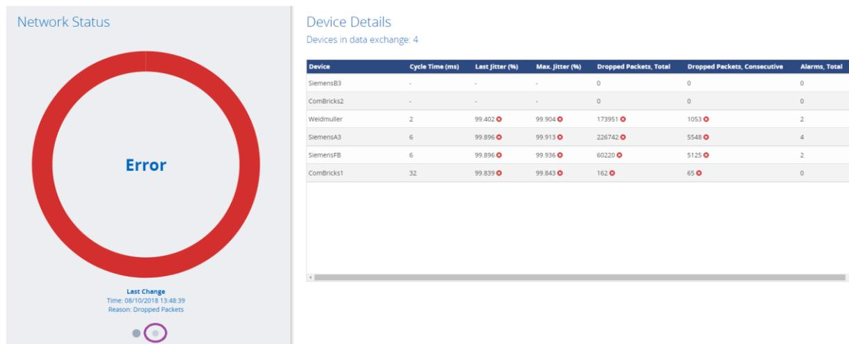
In case of errors, the large circle turns red as shown in the image. The right pane is a list of PROFINET statistics and errors per device.
